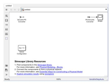
By default, the model name is not specified, the model contains a Solver Configuration block, a Simulink-PS Converter block, and a PS-Simulink Converter block connected to a Scope block. The default solver is VariableStepAuto. The resources section at the bottom of the model window provides links to the relevant block libraries and documentation topics.
