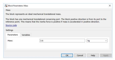
4 To specify the desired initial value for mass velocity, click the **Variables** tab. The **Velocity** variable already has its **Priority** specified as **High**. In the **Beginning Value** field, type 10, then click **Apply**.
