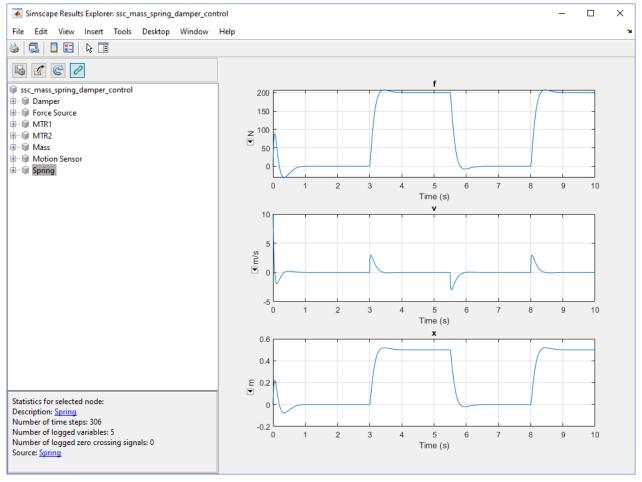
**3** Expand the Spring node and select node x. The right pane displays the spring deformation data plotted over time.
